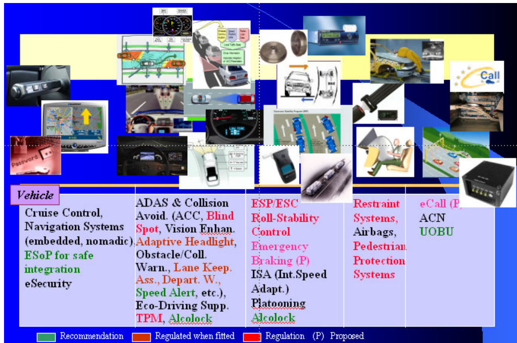
Figure 12: The classification of systems according to the regulation mechanisms (green = recommendations for use, brown = regulated when fitted, red = regulation/mandating, (P) = regulation is planned [picture ACEA])
